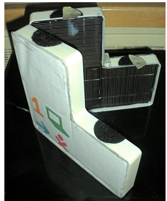
Solar charging device created by first year engineers for a laptop used in developing countries.
